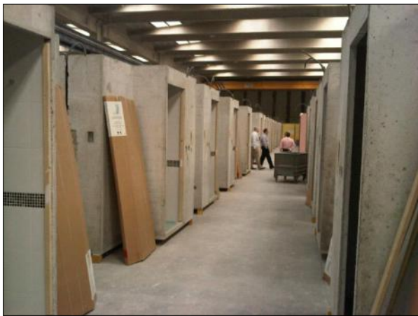
Precast 'Bathroom Pods' in manufacture
